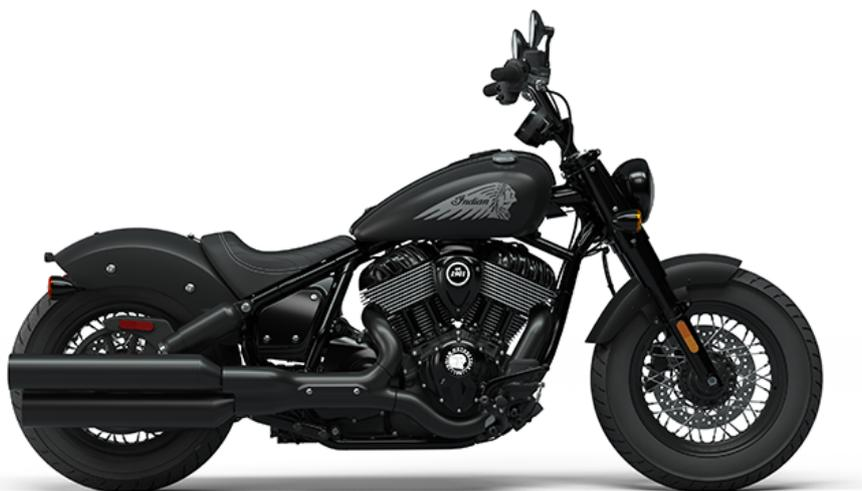
The air-cooled Thunderstroke 116 produces 120 ft-lbs of raw torque for passing power in all 6 gears. It'll catch eyes on the street and grab your soul from the saddle.
